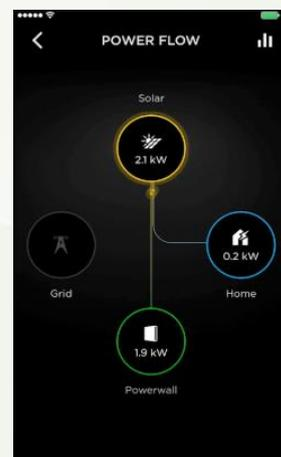
Plate 2: Smart phone App to control personal energy usage, storage and renewables generation (image credit: Tesla Powerwall support)
